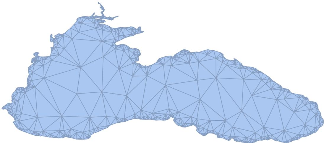
As the triangulation is generated, to each of its nodes (i.e., each vertex of a triangle) and to each element (i.e., each triangle) a number is assigned, as shown below (we shall further use the notation  $\mathbf{N}_1, \dots, \mathbf{N}_N$  for the mesh nodes):
