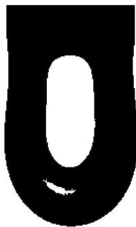
Figure 2.5: Image obtained after step 1 of the edge detection algorithm with \delta = 40 (if \delta is smaller, e.g. 10, we get really curly border) .
