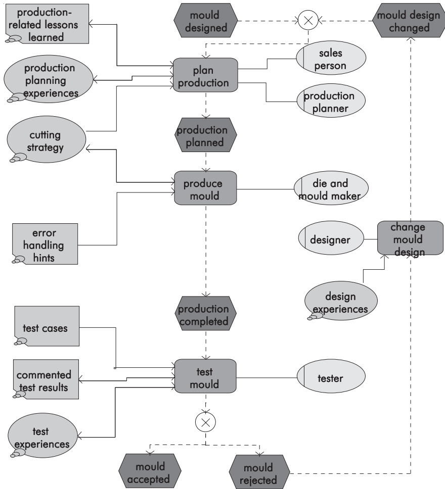
FIGURE B-31. Extended event-driven process chain with KM elements
