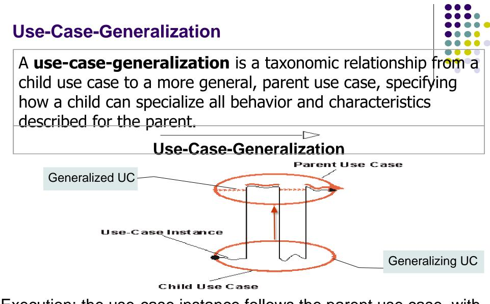
Execution: the use-case instance follows the parent use case, with behavior inserted or modified as described in the child use case. 3. Actors and Use Cases. Diagrams
