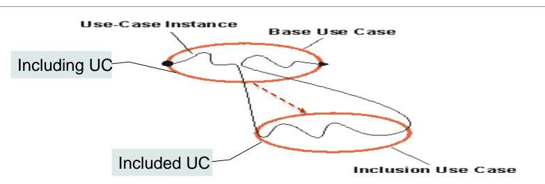
Executing a use-case instance following the description of a base use case including its inclusion. 3. Actors and Use Cases. Diagrams
