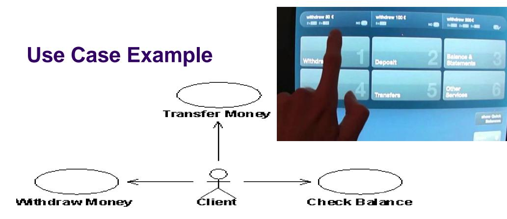
An ATM example - the system functionality is defined by different use cases, each of which represents a specific flow of events, defines what happens in the system when the use case is performed, and has a task of its own to perform.
