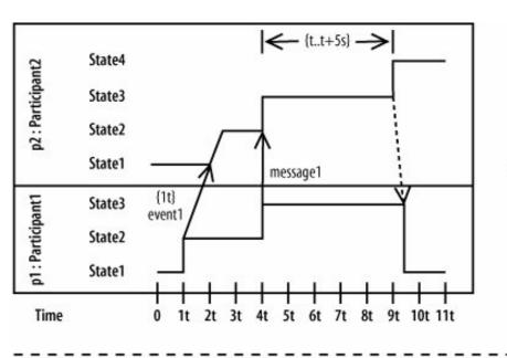
The regular Timing Diagram notation: good when fewer states need to be shown.
