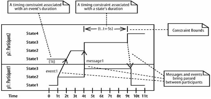
Timing constraints can be associated with an event or a state and may or may not be accompanied by constraint boundary arrows
