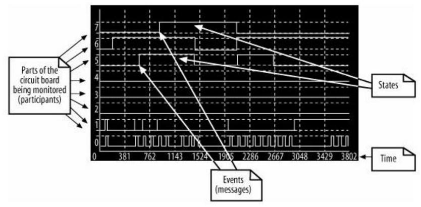
A logic analyzer captures a sequence of events as they occur on an electronic circuit board
